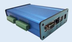
⇒ **Axion Device Application**: Following figure is an Axion OEM-2100 which includes a set of gas analyzers, an engine diagnostic, a GPS, a EFM, and embedded software. The gas analyzers measure concentration of NOx (NO and NO2), HC, CO, CO2, and oxygen(O2) in the vehicle exhaust. User Interface (UI) using Windows Form Application with XML and C# is created to display data on the monitor of the Axion device.
