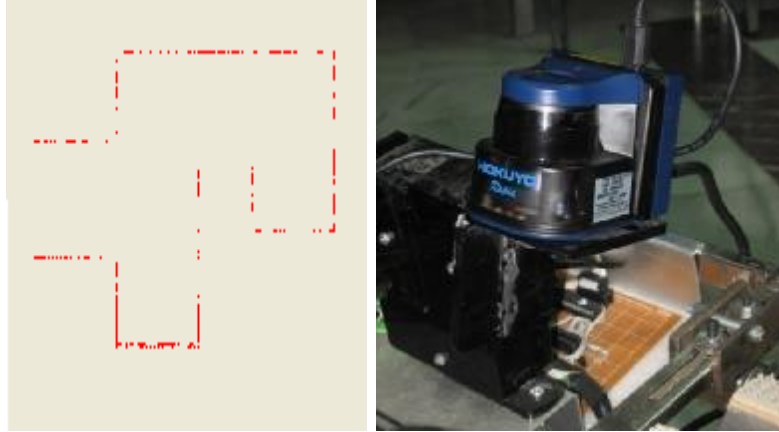
Fig 8 laser scanner (Hokuyo UBG-04LX-F01)
