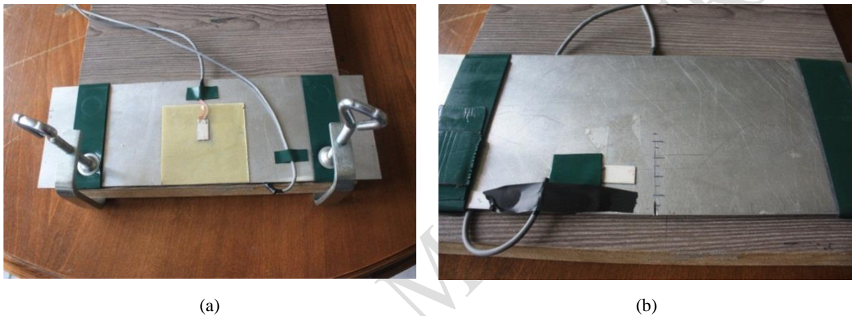
Figure 5. (a) Top view: Sensor attached to the composite patch; (b) Back view: Sensor attached to the metal and crack propagation path
