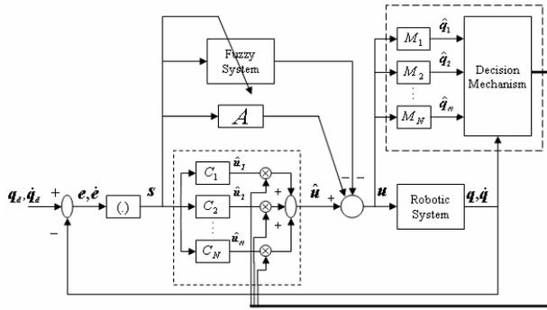
Fig.1 Adaptive fuzzy sliding mode control using multiple models approach
