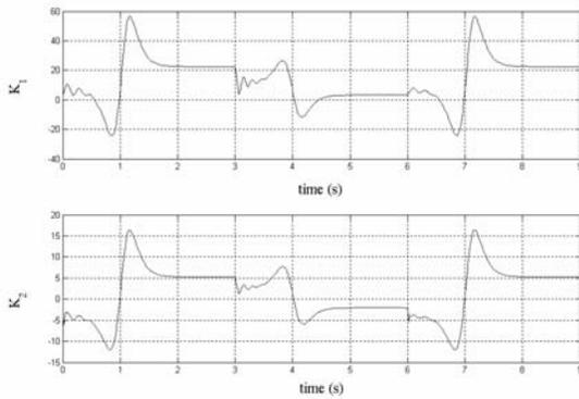
Fig.4 Control gains of joints 1 and 2 (outputs of fuzzy systems).
